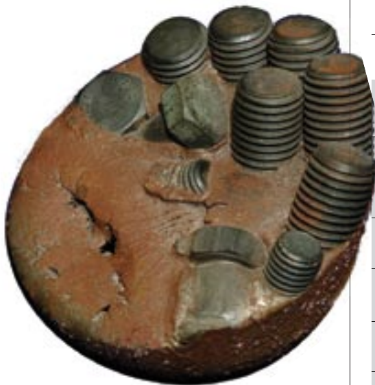
Stainless-steel melt demonstrates energy-efficient microwave melting techniques
