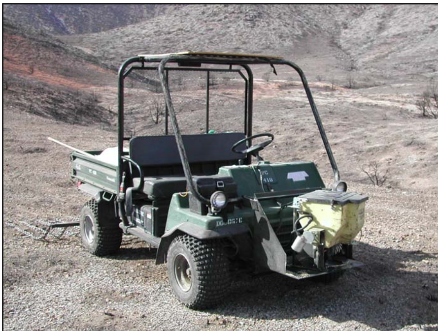
Figure 6-5. An all-terrain vehicle with a mechanical seeder attached to the front and drag chains on the back was used to seed the lower slopes and bottom areas of the Egg Point Fire burn site. (Photo by D. Anderson, January 28, 2003).
