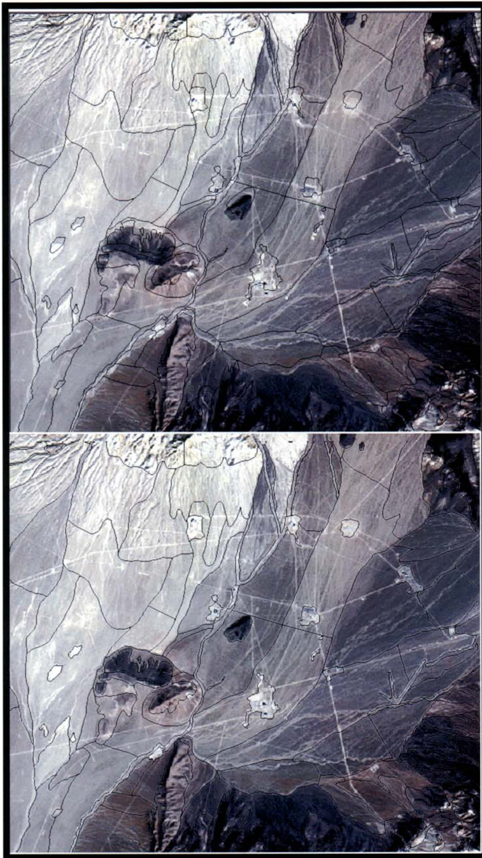
Figure 4. Example of inaccurate registration of ELU polygons with orthophotos in Jackass Flats (upper photo) and accurate registration after spatial adjustments were made (lower photo).
