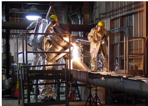
NETL-Albany employees recovering precious metals from catalysts via water-jet granulation of molten metal.
