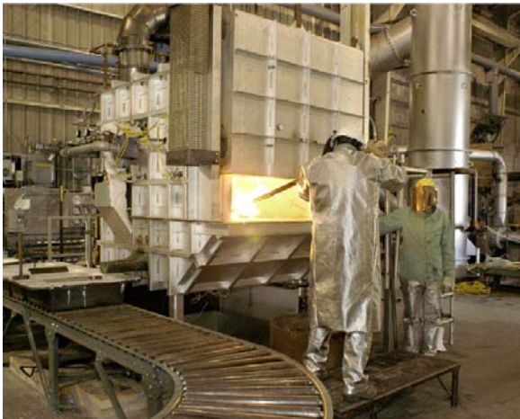
NETL-Albany employees removing dross from an aluminum melting furnace.
