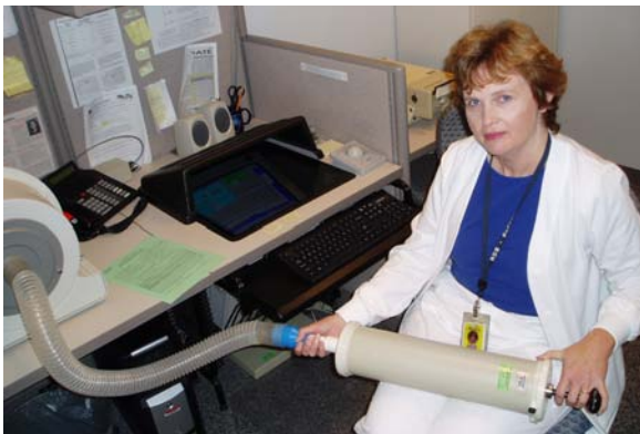
Trisa Pew calibrates a Spirometer in the Occupational Health Unit at NETL.
