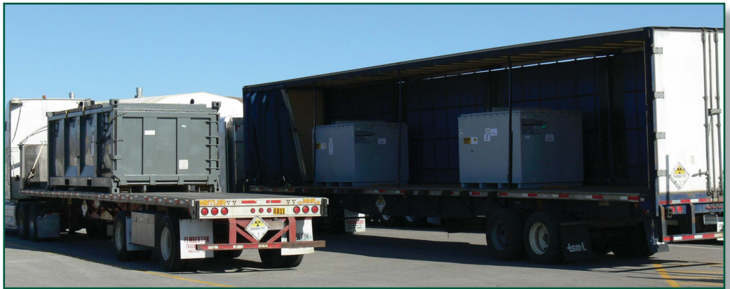
Waste packages are transported to the NTS on a variety of tractor trailers. The load securement devices which stabilize waste packages during shipment are removed and any curtains of enclosed trailers pulled back in preparation of a radiological survey and off-loading by NTS Disposal Operations personnel.
