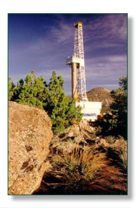
Wells are drilled to collect groundwater samples, which help scientists determine contaminant boundaries and movement.
