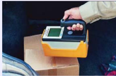
Using a RIID to determine if material is illicit
