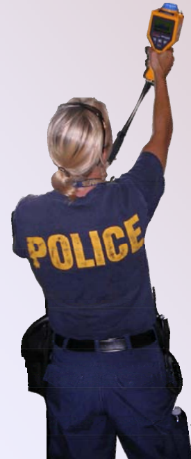
Officer locating radioactive material with a RIID
