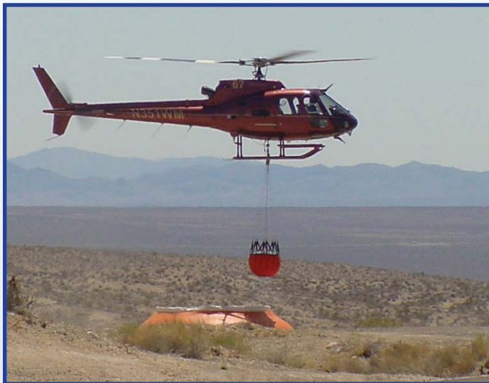
Helicopters are used during wildland fires at the NTS to make 120-gallon water drops on hot spots.
