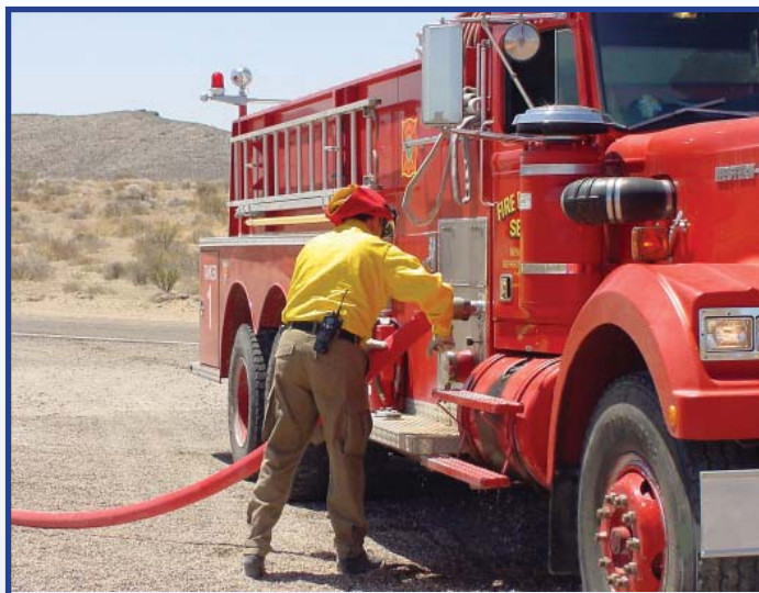
NTS Fire & Rescue equipment includes an engine containing a 1,250 gallon-per-minute pump and 1,000-gallon tank.
