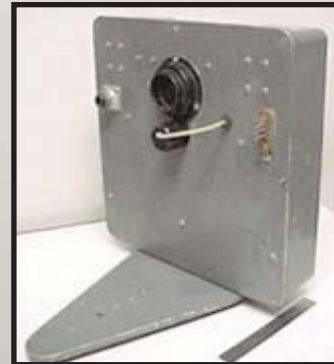
Because the rapatronic camera could only take one photo, banks of cameras were needed to photograph a single nuclear test.
