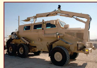
Buffalo Mine Protection Clearance Vehicle detects improvised explosive devices patrolling in Baghdad, Iraq.
