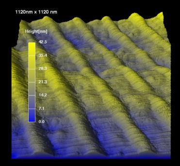
Perspective view of the AFM-topographical image of a planaraligned Wacker OCLC . 1120 nm x 1120 nm scan.
