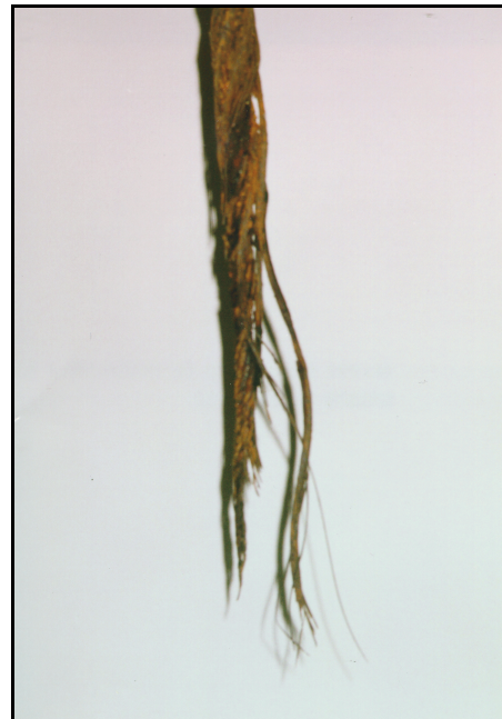
Figure 4.—Stewart Mountain Dam broken wire rope.
