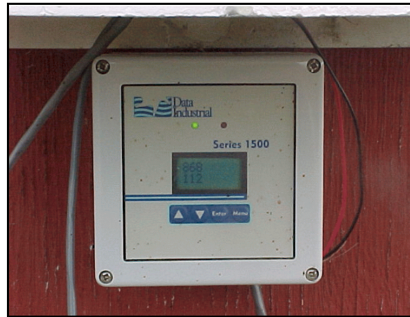
Figure 6.—The display for the paddle wheel sensor in figure 5. The top number displays gallons per minute, and the bottom number displays total water in cubic feet.
