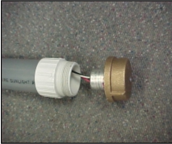
Figure 9.—Pressure transducer threaded into a pipe cap prior to attaching the cap to the end of PVC tubing.
