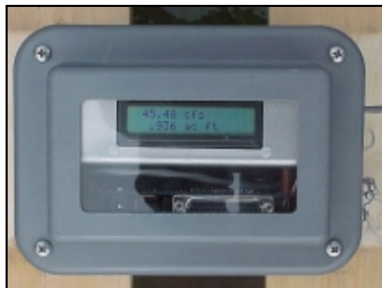
Figure 2.—View looking down on top of the flow recorder showing the readout in cubic feet per second and total flow in acre-feet.
