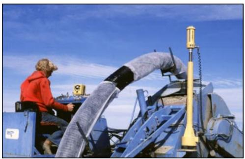
Figure 3.—Pipe with thin filter sock.
