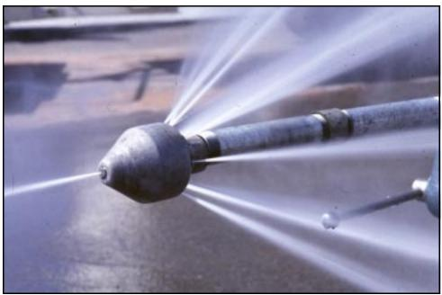
Figure 14.—High-pressure spray nozzle.
