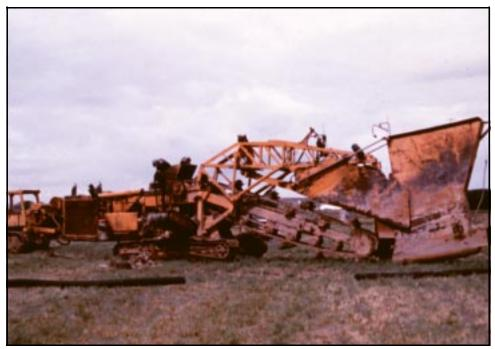
Figure 8.—Ladder trencher.
