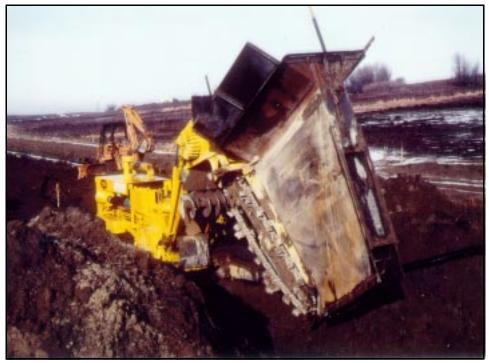
Figure 9.—Chain trencher.
