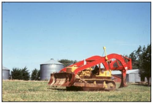
Figure 11.—Drain plow.
