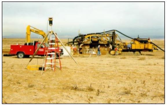
Figure 12.—Laser plane system.
