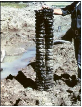
Figure 1.—Pipe failed due to stretch.
