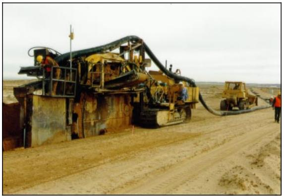
Figure 7.—Wheel trencher.
