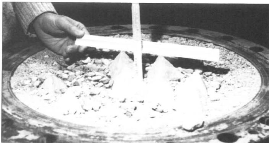
Figure 1.—Simulated substrate in the puncture test.
