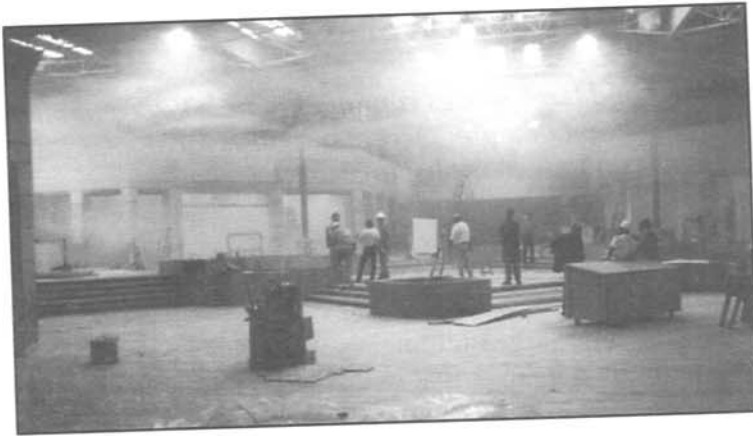
Warm smoke from test rig results in a smoke layer well above the occupied level, providing acceptable visibility and tenable conditions throughout the egress path. (Photos provided by Carl Baldassarra, Schirmer Engineering.)
