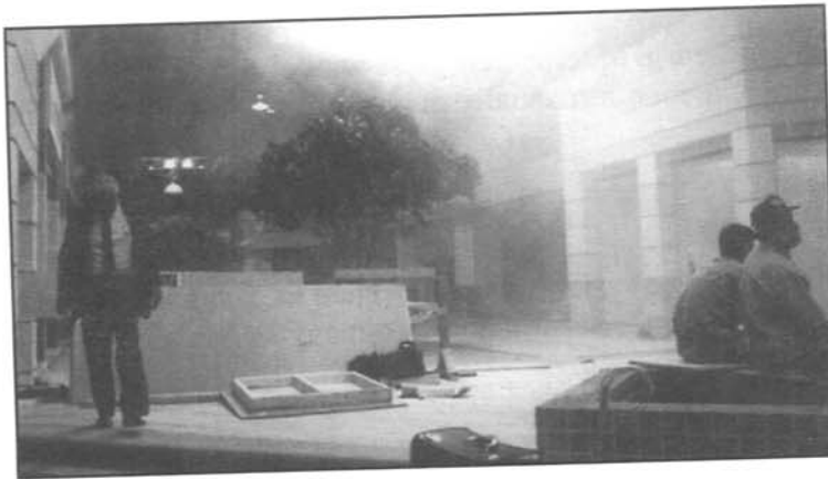
An unanticipated high-velocity air pattern has drawn air from the smoke layer down to the occupied level at right, hindering egress travel in that area. This disturbance could be corrected before occupancy because it was identified by the smoke rig testing.
