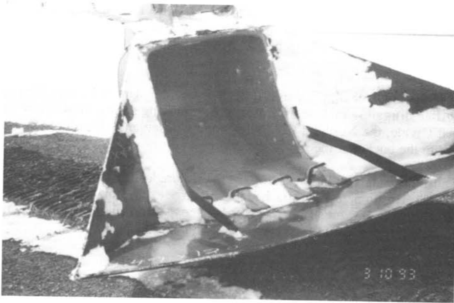
Photo 2. – Bucket attachment installed to make “Grand County Dipper.”
