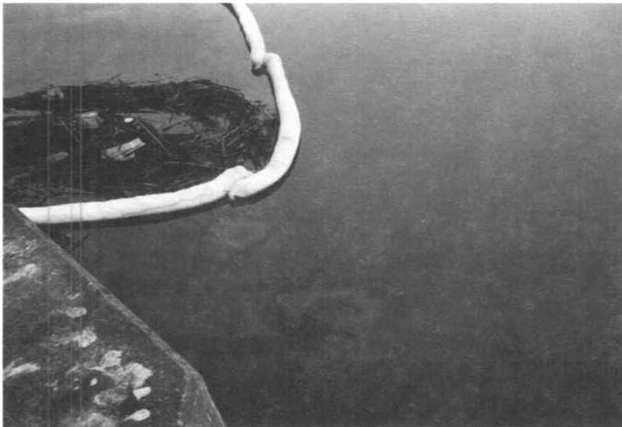
Photo 14. - Intake channel—oil boom, film going under because boom on top of some debris. 1/18/91
