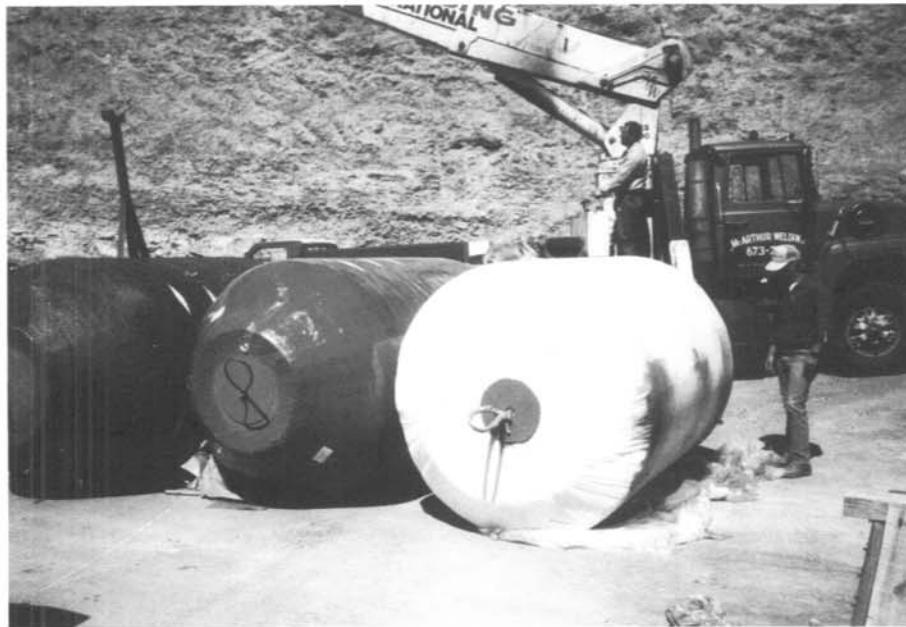
Left to right, 66-inch pigs: (1) pig with urethane coating embedded with carbide chips, (2) pig with urethane coating only, (3) lightweight foam pig.
