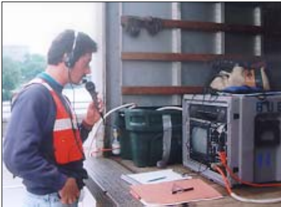
A dive team leader communicating with the inspection diver during underwater inspection being documented on videotape.
