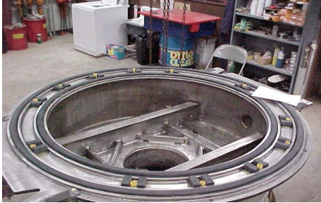
Bulkhead seal system before seals were installed.
