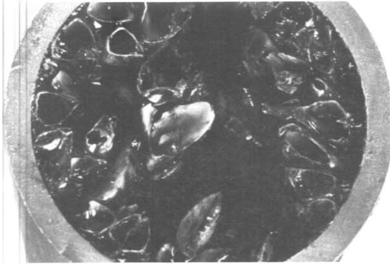
Photo 2.—Small floating larvae of zebra mussels are drawn into water intake pipes where they settle down, grow, and block waterflow to critical components of cooling systems in industrial plants and on ships and pleasure boats. (Photo by Peter Yates)
