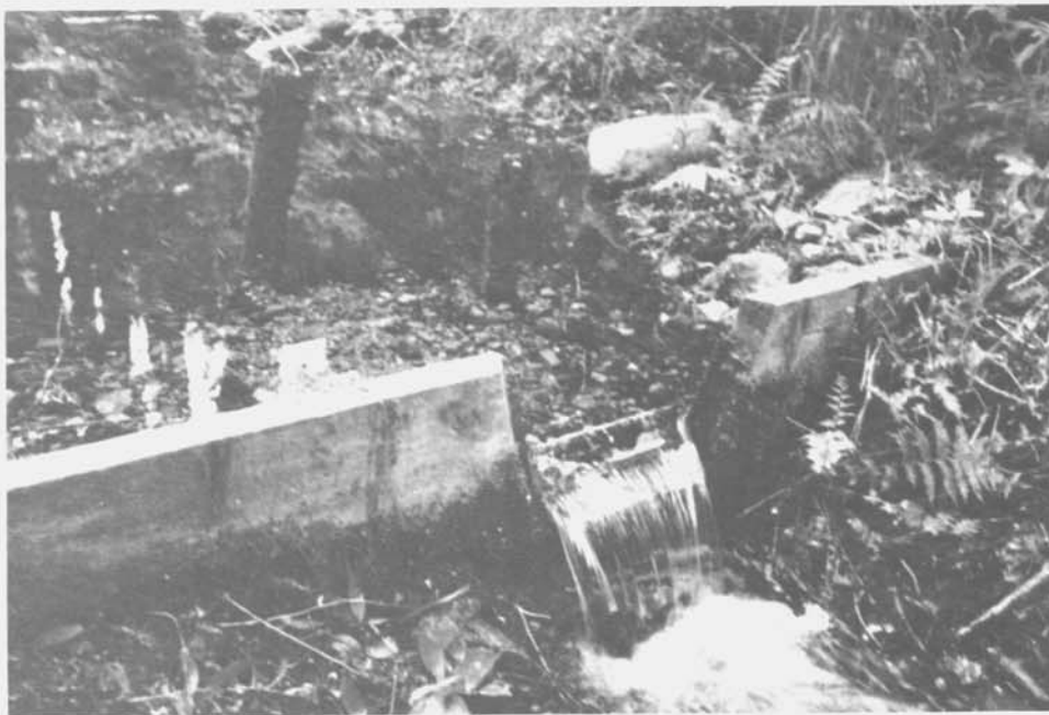
Figure 4.—Measuring devices, such as shown above, are a simple and economical means of monitoring seepage at the dam. Records should be kept of all significant activities, such as this, at the dam and entered into the operating log as a permanent record.
