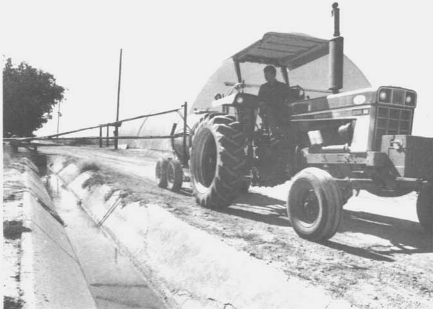
Figure 8.—Williams' ditch sprayer allows the operator to either spray ditchbanks and turnrows separately or together.
