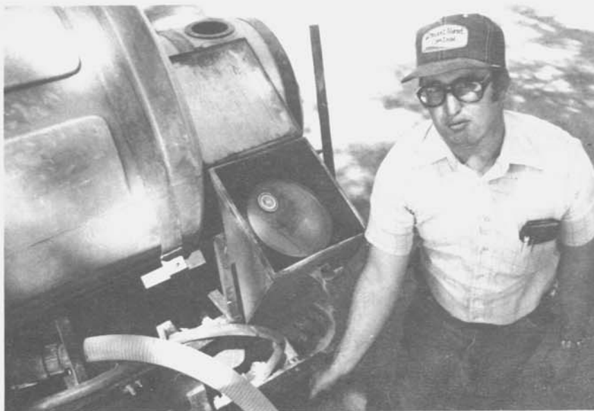
Figure 5.—A feature of the Gable tank truck is the closed system used to transfer chemical from 19 L (5 gal) cans into the water-filled tanks. The closed system will not only open cans but will triple rinse them as well.
