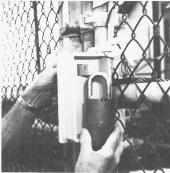
Figure 4.—Camaloy chain and high-security padlock.
