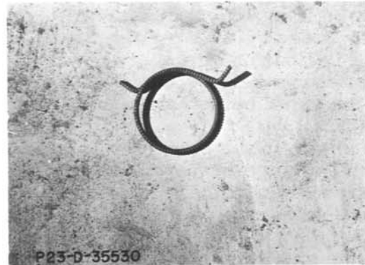
Fig. 2--Re-bar ring made with bender.
