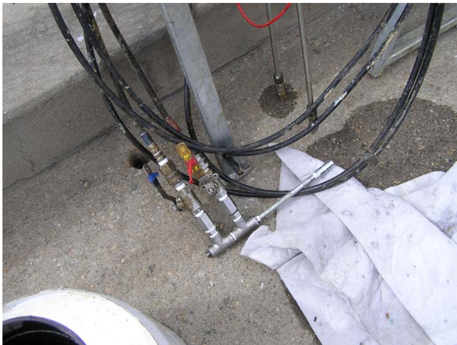
"F-assembly" injection gun.
