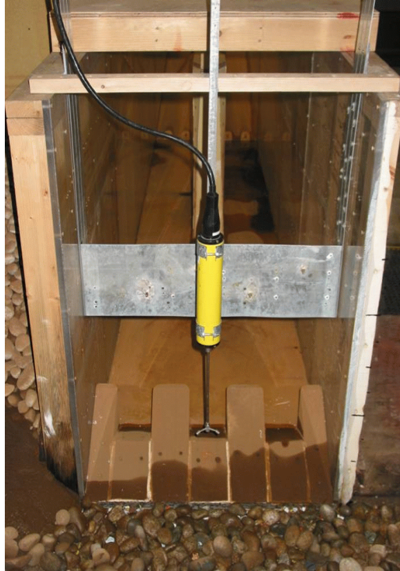
Figure 4.—Looking upstream at stilling basin model with ADV probe and deflector installed near the end of basin.
