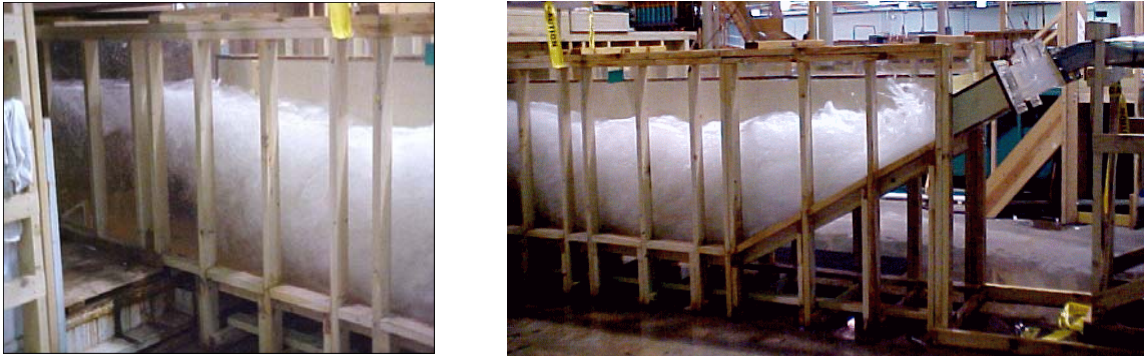
Figure 3.—Looking through the plexiglass sidewall of the model operating at 40 percent gate opening.
