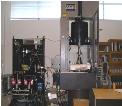
Stiff testing frame.
