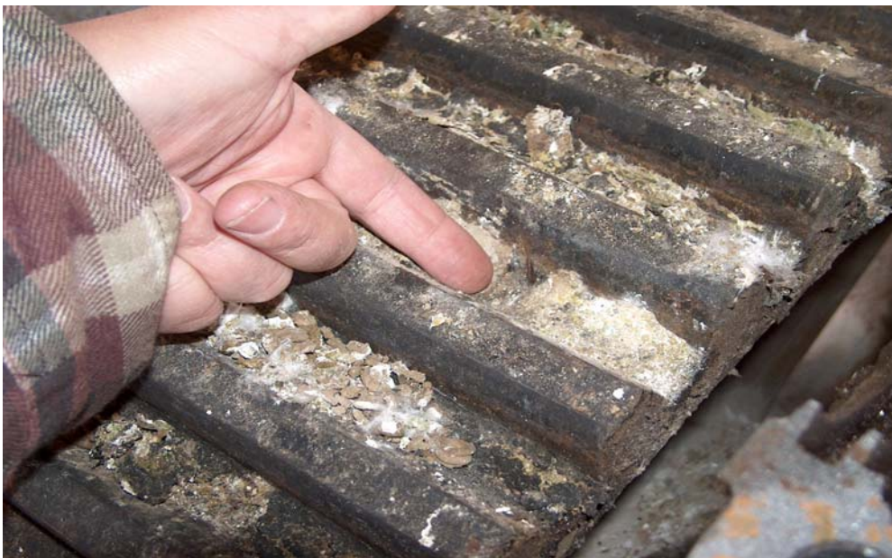
Photo 2.—Debris in gear teeth.
