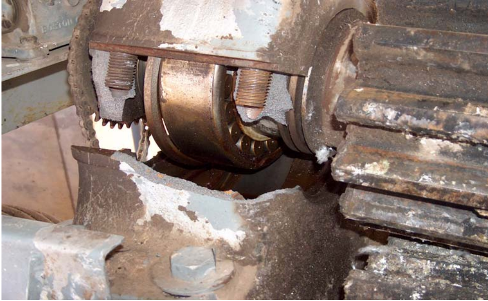
Photo 1.—Fractured casting – pillow block bearing (Part 42).
