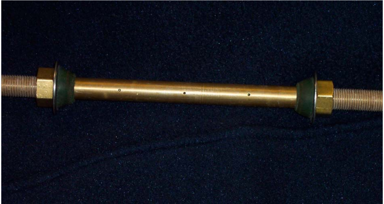
Figure 1.—Prototype Mag-tube flow meter, with three pressure taps on the upstream side of the tube.
