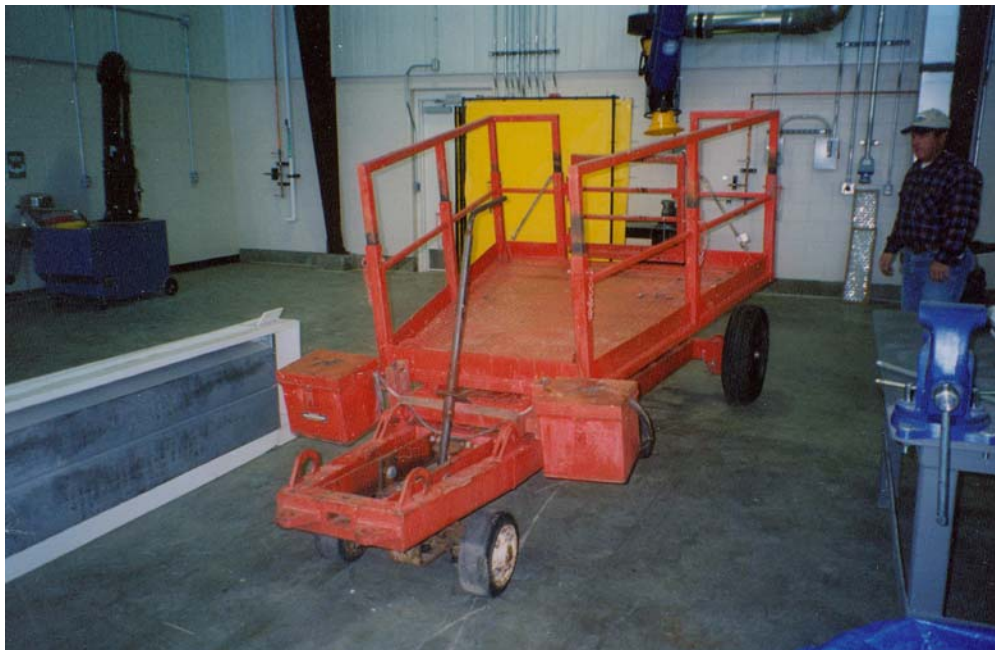
Photo 3.—Cart, which has been modified to allow steering (to keep it from crawling up the sides of the conduit). The hoist cable attaches to the “steering” end of the cart, and the cart is lowered down the steep slope of the siphon.
