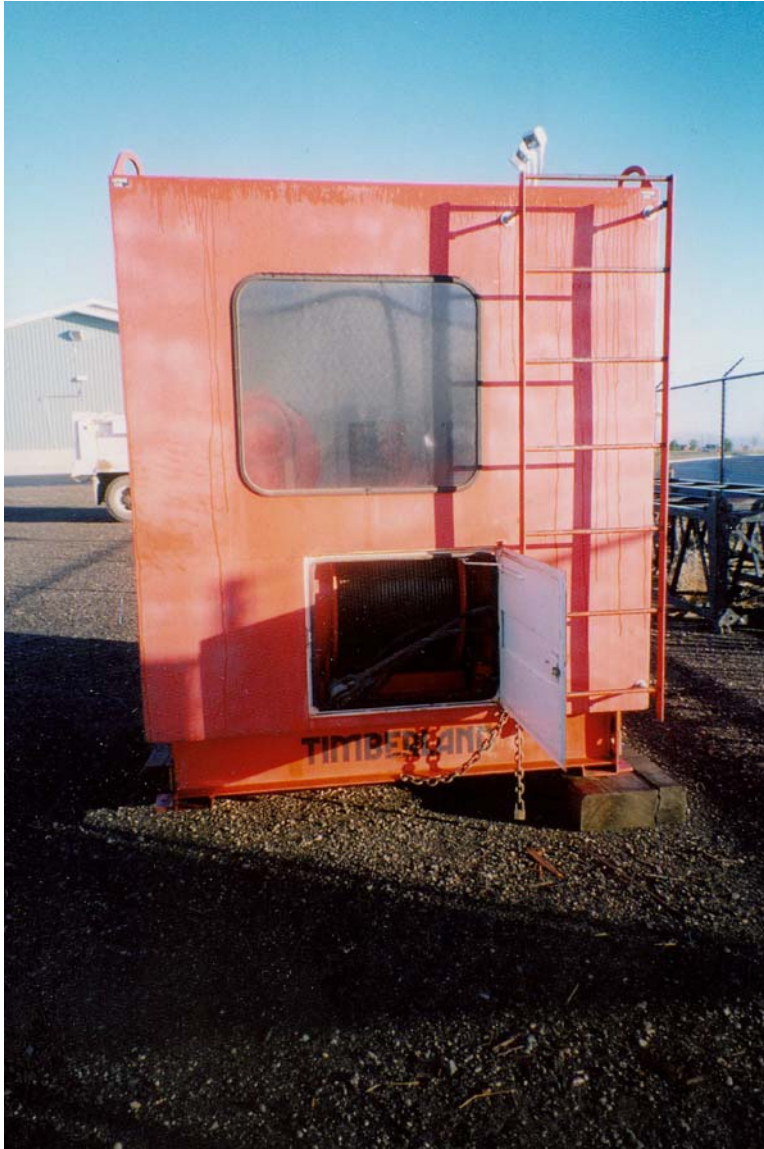
Photo 2.—Personnel and material hoist unit (exterior of unit, looking toward operator). The cable drum is visible through the open door. The hoist is placed in the canal near the entrance to the siphon.
