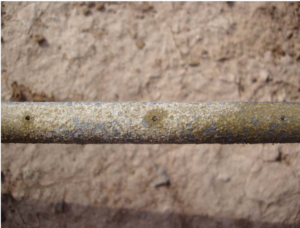
Figure 5.—Scale formation on aluminum Mag-tube.
