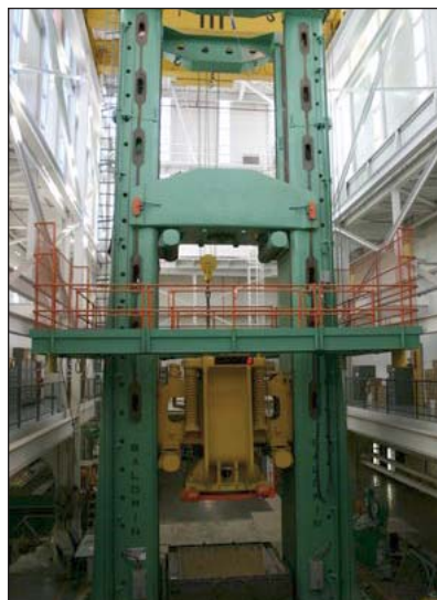
The five million pound press is used to test the strength of concrete and other materials. It is one of the tools the Technical Service Center uses to support the Reclamation mission.
