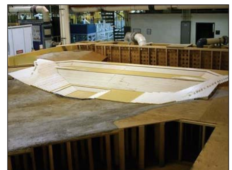
Scale models are used in the Technical Service Center's Water Laboratory to see how modifications affect the movement of water through Reclamation's facilities.
