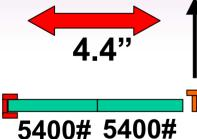
There are only pallet locks between IATA position 22L&R and 23L&R! You must accept a 4.4" gap with a "stack" of only 2 LD-8s, 2 LD-3s, or 4 LD-2s here.
