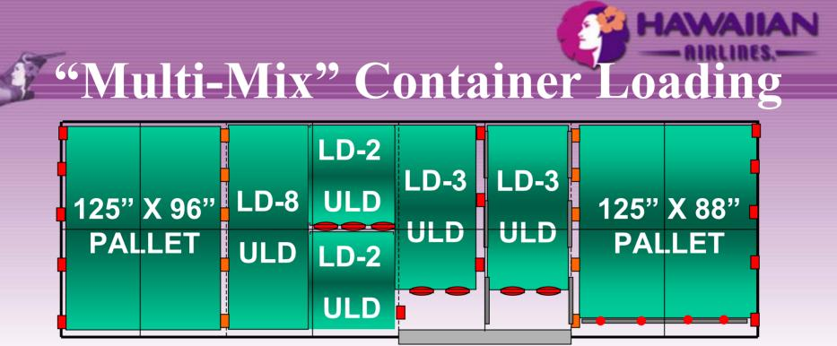
The ability to load various types of pallets and containers comes with a price...accommodation requires a compromise between location and type of restraint hardware...resulting in restraint of groups or "stacks" of containers vs. individual ULDs (our previous experience with the DC-10).
