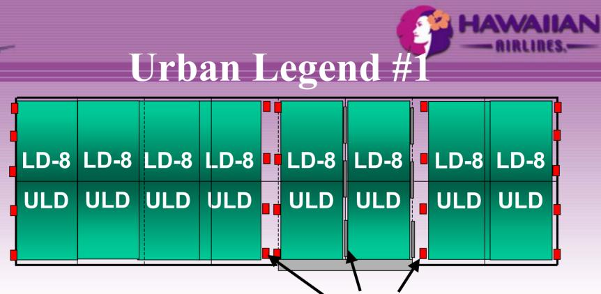
"Please advise the loaders that certain latches need to be set <u>even if the hold is a full fit</u> to reduce gaps, which can cause noise, triggering false alarm load shifts."
