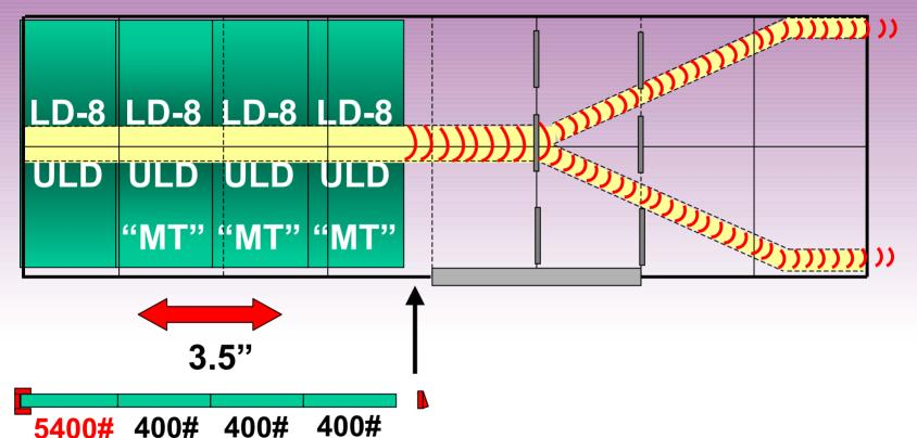
Why does the noise sound like it's coming from directly behind the cockpit? One theory – empty cans act like a bellows...a large ventilation duct below the cargo deck transmits sound waves.
