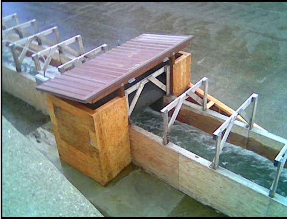
Photo 5. PIT tag antenna showing enclosure, sun shade, and spillways flow deflector
