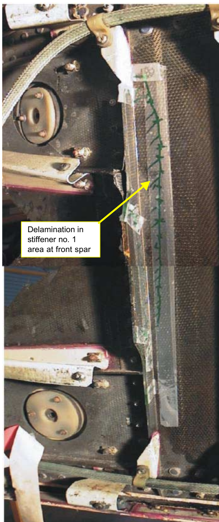
Photo no. 01: Delamination at front spar; stiffener no. 1
