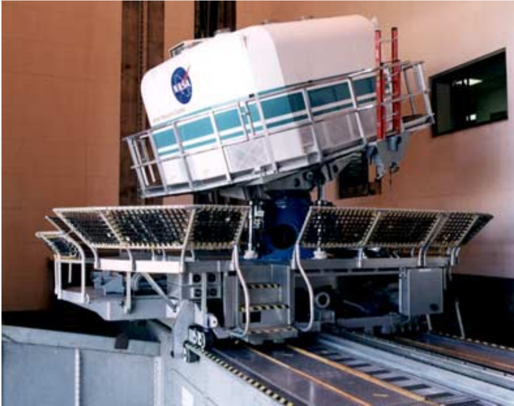
Figure 1. The NASA VMS cab and motion platform.
