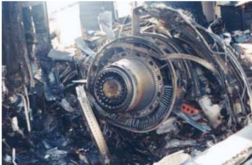
Photo 4: No. 2 engine's core separated from fan
