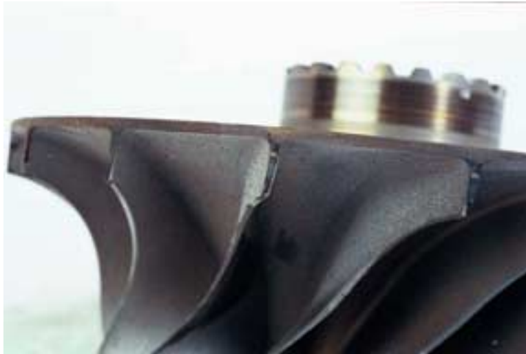
Photo 28: Close up of 1 st stage impeller showing no circumferential rub marks (Honeywell)
