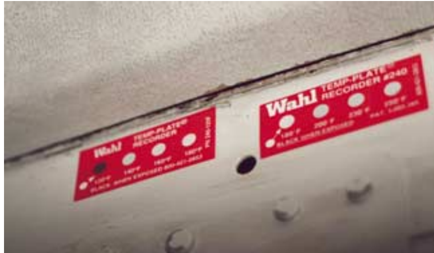
Photo 34: Temp tabs on frame C83 showing exposure to 120°F
