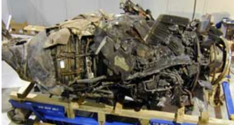
Photo 18: As received condition of No. 2 engine minus the fan (American)
