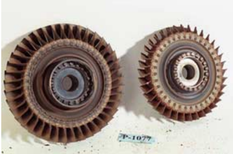
Photo 30: 1 st and 2 nd stage turbine disks showing no bent blades (Honeywell)
