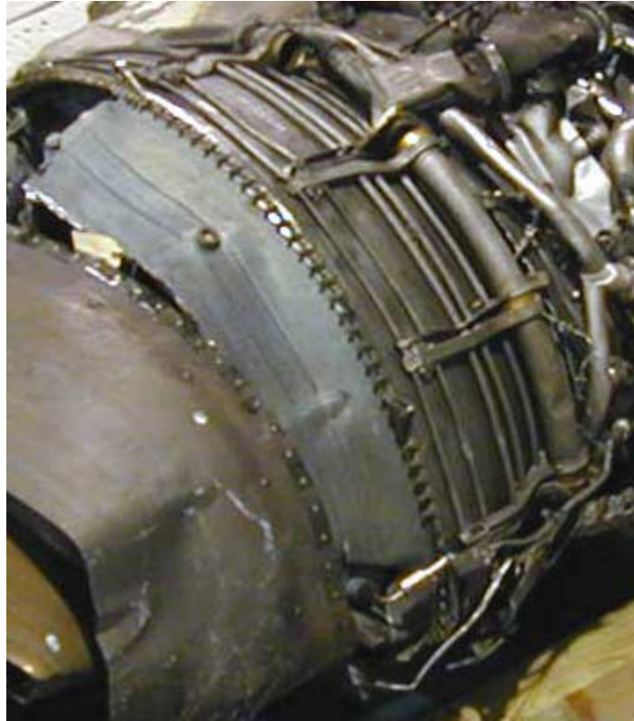
Photo 15: No. 1 engine's low pressure turbine case and the broken turbine rear frame (American)
