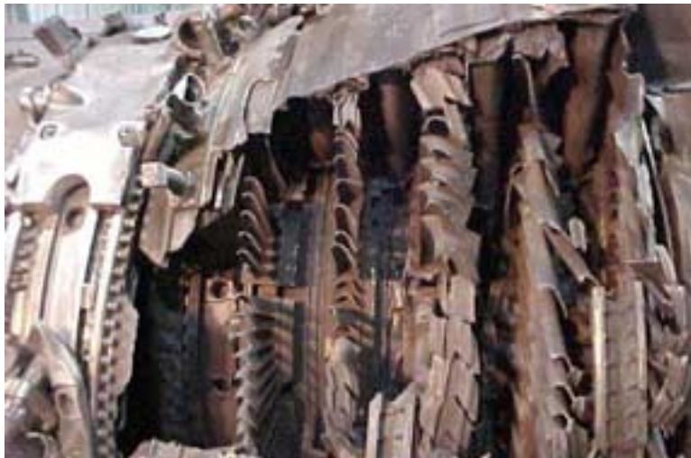
Photo 16: No. 1 engine's low pressure turbine case cut away exposing blade and vanes (GE)
