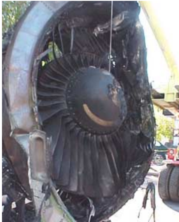
Photo 5: No. 2 engine's fan blades shown after fan had been picked up (FAA)
