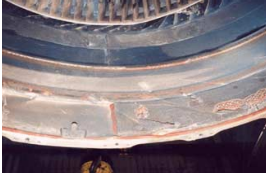
Photo 9: No. 1 engine's fan case and rub strip showing imprint of fan blade tips
