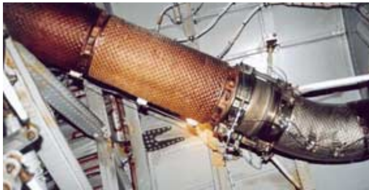
Photo 33: Example of APU bleed air duct exiting firewall in tailcone showing overheating detection wires in American Airlines A300 N70054
