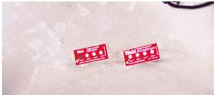
Photo 36: Temp tabs on vertical stabilizer access cover showing exposure to 120°F
