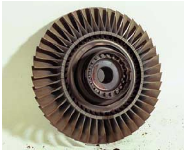
Photo 31: 3 rd stage turbine wheel (Honeywell)
