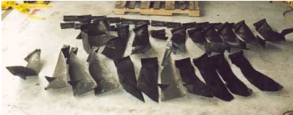
Photo 20: No. 2 engine's fan blades
