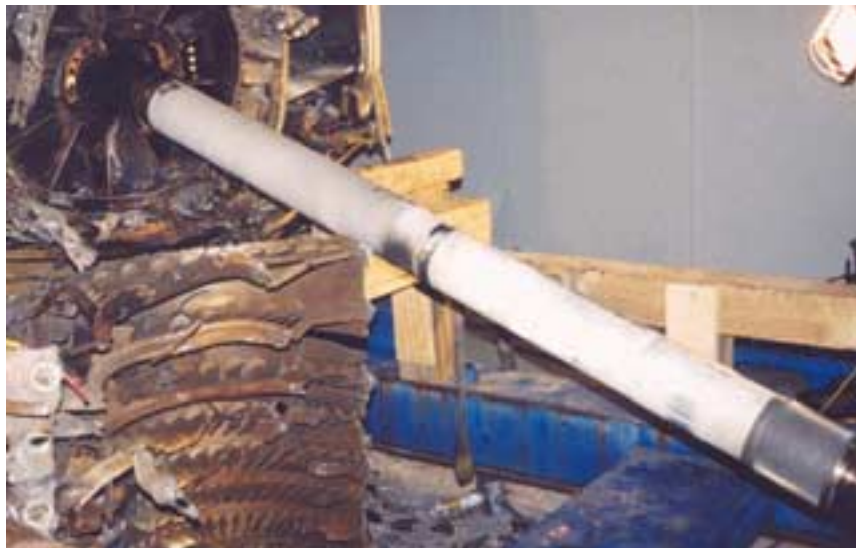
Photo 11: No. 1 engine's fan mid shaft
