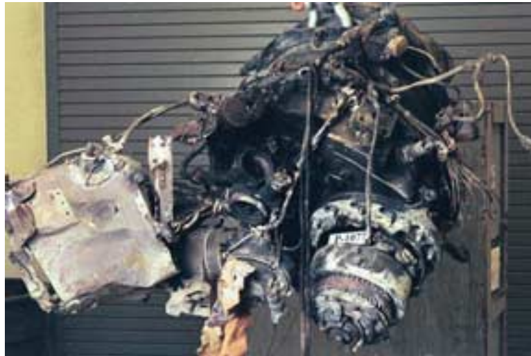
Photo 32: Gearbox and load compressor broken away from APU power section (Honeywell)
