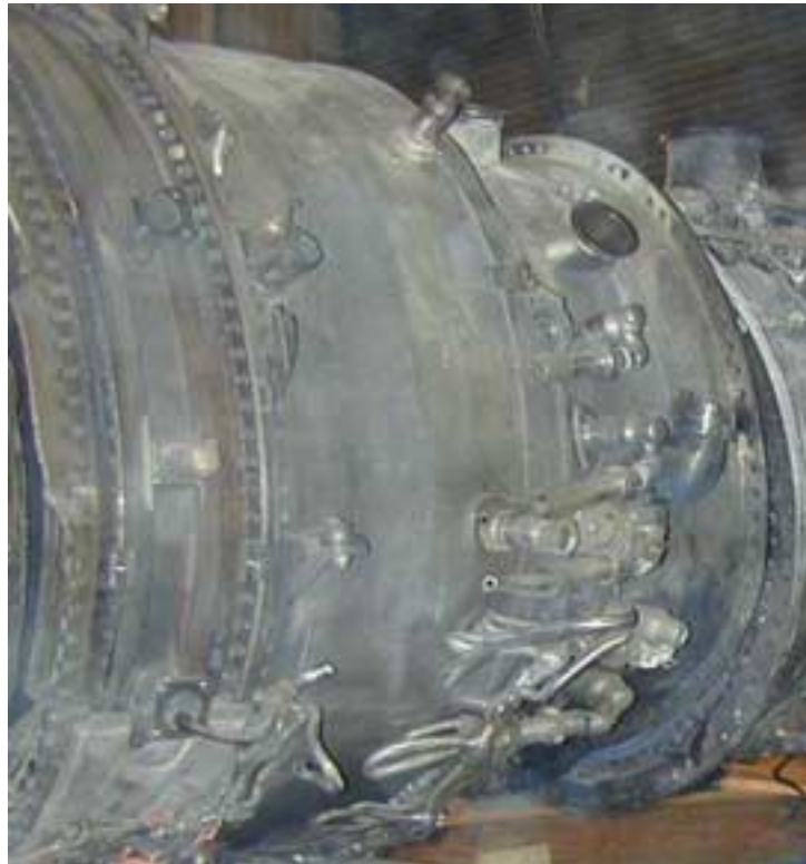
Photo 13: No. 1 engine's compressor rear frame (American)
