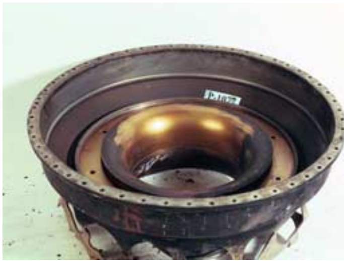
Photo 29: 1 st stage impeller shroud coated with soot and where soot was wiped away, no impact marks from the impeller (Honeywell)
