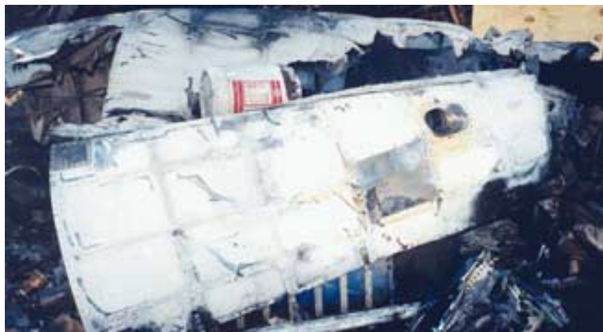
Photo 7: Tailcone over area of APU installation showing no shrapnel damage
