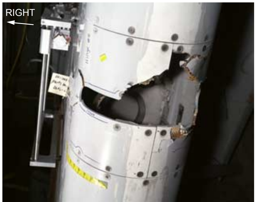
Figure 53. The LE fairing at hinge 5 as viewed looking mainly down and aft. Lamb wave equipment used for nondestructive examination is shown in the background on the right skin panel.
