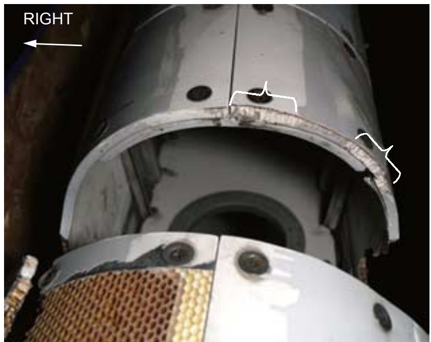
Figure 58. View of the upper side of the hinge 7 LE fairing cutout. Brackets indicate areas of damage on the left side.
