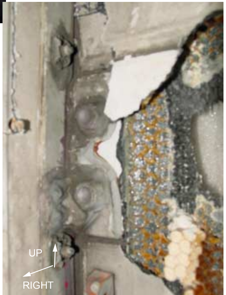
Figure 33. View of the right side hinge 2 aft fitting piece that remained attached to the rudder.
