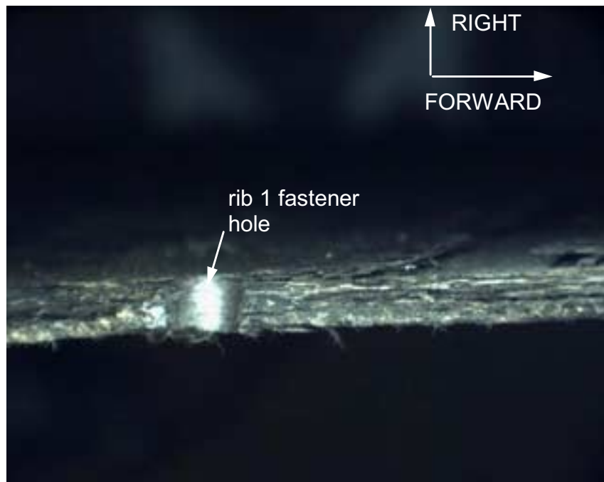
Figure 32. Vertical stabilizer skin fracture at a rib 1 fastener hole in the vicinity of the left aft lug, viewed looking upward.
