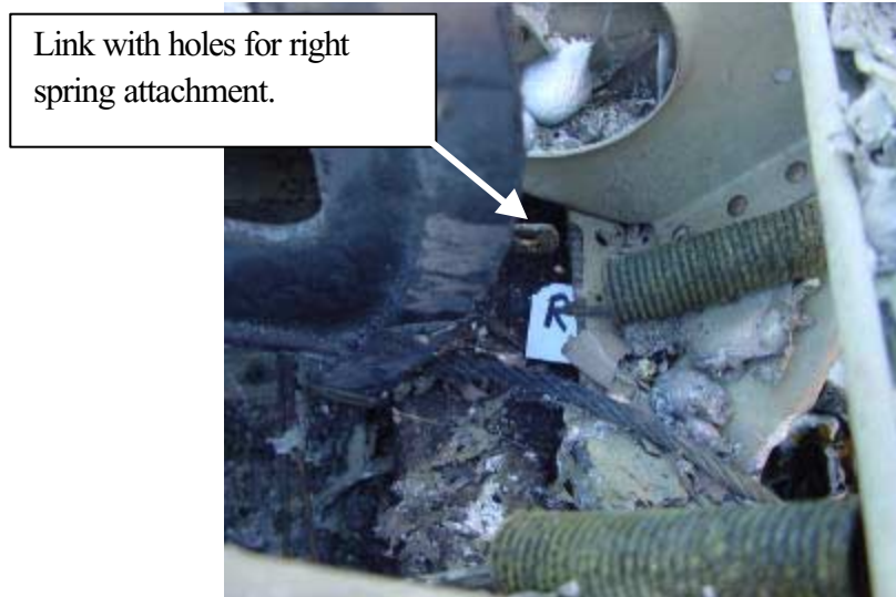
Photograph 7. Left and right springs shown, right spring is not attached to link. (Right edge of photo is toward nose of airplane.)
