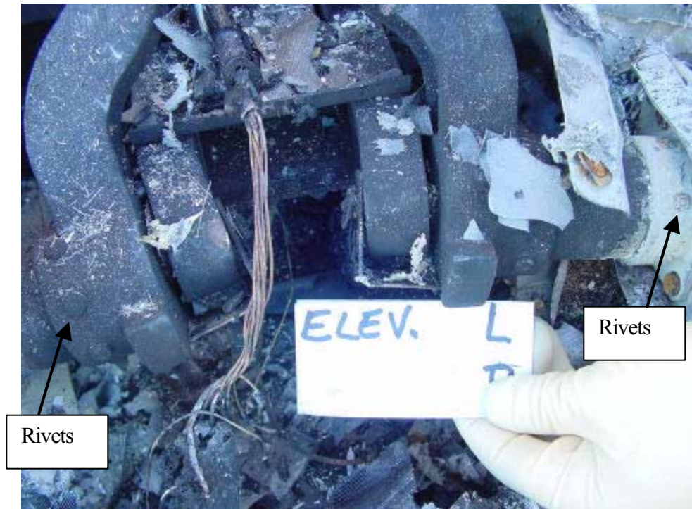
Photograph 1. Elevator control horns- left and right elevator
