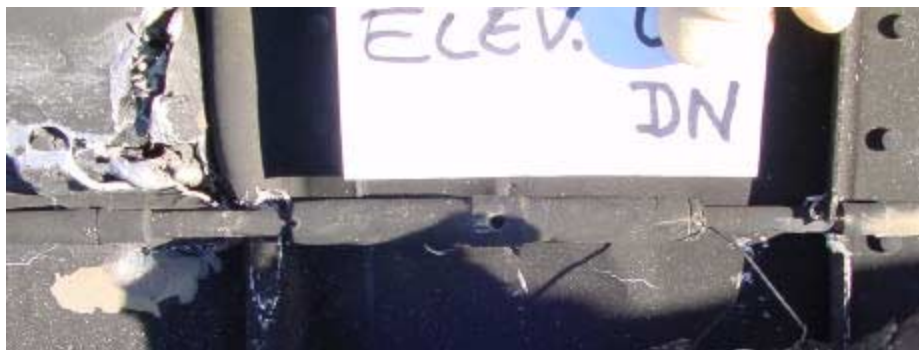
Photograph 9. Elevator “AND” cable turnbuckle. Note: this turnbuckle was pinched in structure and the safety clip that is visible beneath the “DN” lettering was pulled off during extrication. To mark the rotational position, a stripe of gloss black paint was applied.
