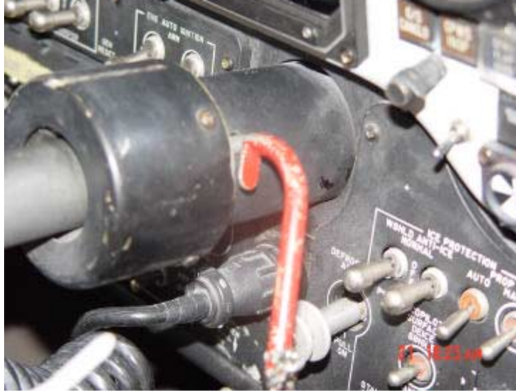
Photograph 12. View of a gust lock installed to immobilize pitch controls in a Model 1900D. (The accident airplane is not shown in this photograph.)
