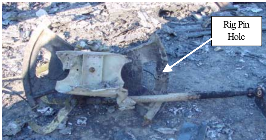
Photograph 6. Aft bellcrank after removal, laying inverted, with right side visible.
