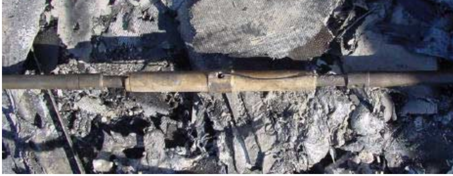
Photograph 10. Elevator “ANU” cable turnbuckle
