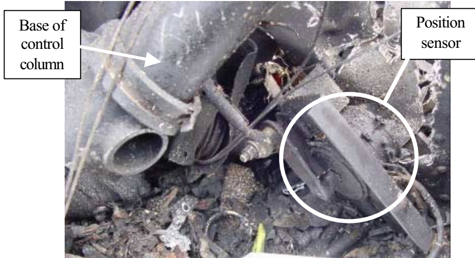
Photograph 14. Column, position sensor, clamp, and linkage.
