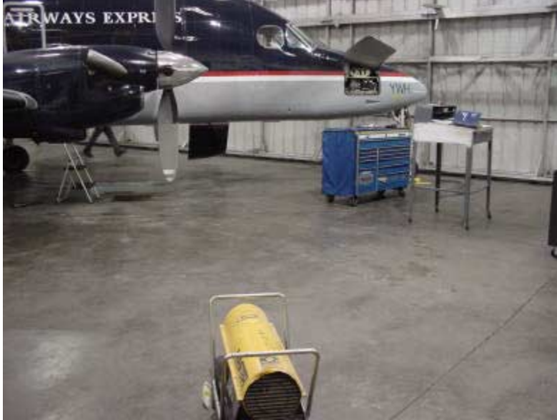
Photograph 2. Kerosene-burning heater pointed toward the right side of the airplane, ahead of wing. Master Model B110BT with placarded output of 110,000 BTU. Note: The location for the OAT probe is on the opposite side of the airplane, beneath the Captain's side window.
