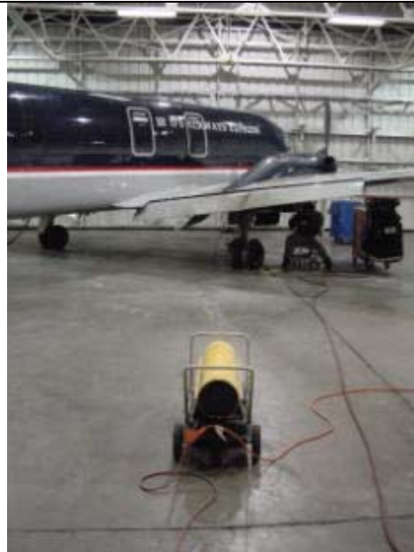
Photograph 4. Kerosene-burning heater pointed toward the left rear of the airplane. Master Model B110BT with placarded output of 110,000 BTU
