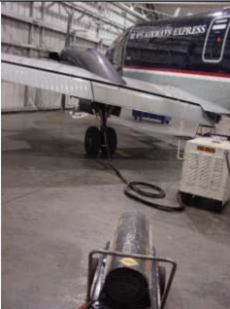
Photograph 3. Kerosene-burning heater pointed toward the right rear of the airplane. DESA Heater Model REM150B with placarded output of 150,000 BTU.
