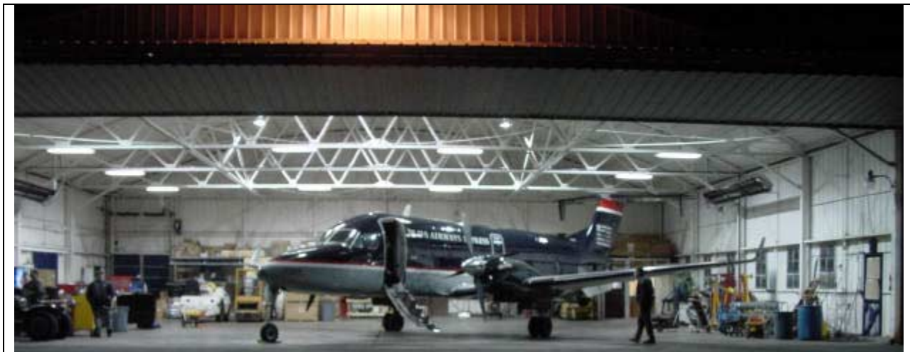
Photograph 1. The photograph shows the hangar before the door was lowered, the airplane parking position, the location of OAT sensor (beneath Captain's side window), and the two heaters between roof trusses of the hangar. The portable heaters had not yet been placed, although one is visible (yellow) to the left of the nose tire and a (black) second portable heater is behind the knee of the person walking. This is not the accident airplane.
