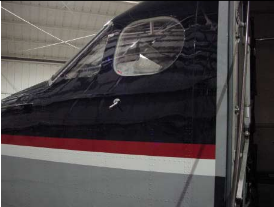
Photograph 5. Installed OAT gauge, beneath Captain's side window. The air-stair is at the right edge of the photograph.
