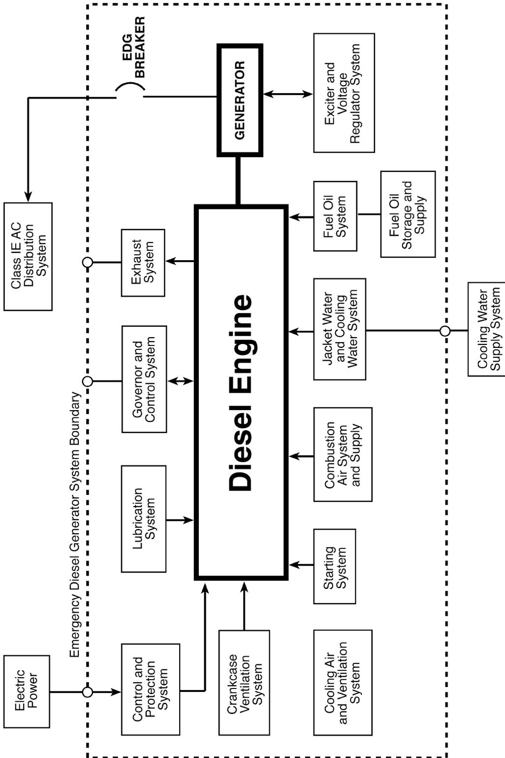
Figure 1. Boundary and Support Systems of Emergency Diesel Generator Systems
