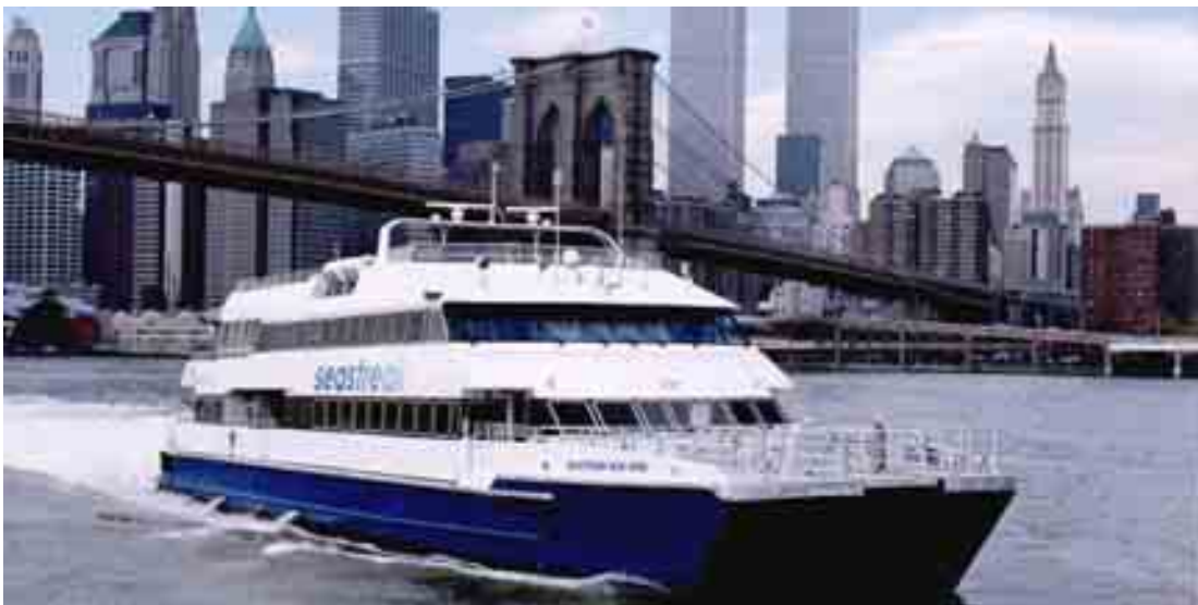
Figure 1. The Seastreak New York is one of a growing number of high-speed passenger vessels in use as commuter ferries. It had a capacity of 394 passengers.
