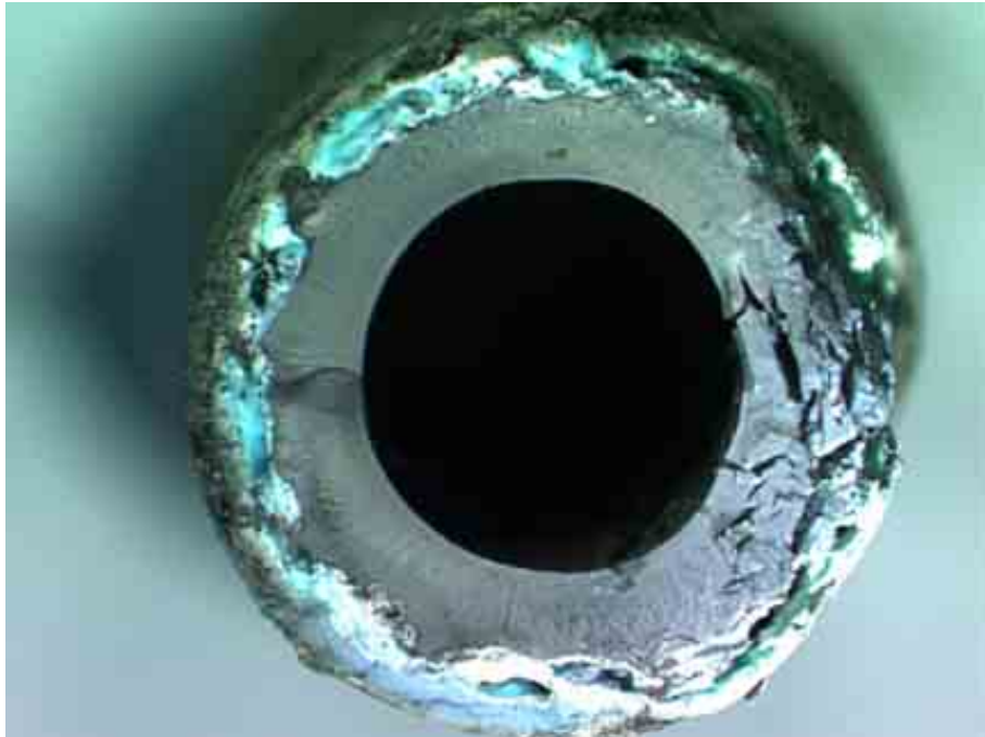
Figure 4. The fracture face of engine No. 3's lube oil monitor hose.
