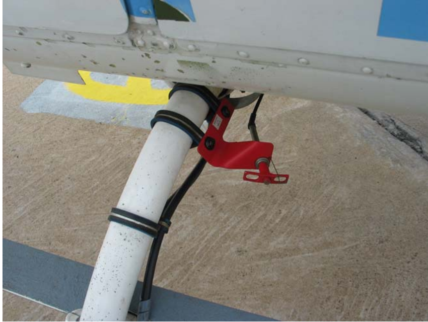
Figure. An external liferaft T-handle on a Bell 206 helicopter forward cross tube
