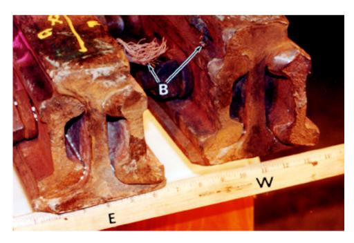
**Figure 6.** The accident joint bars. The east and west sections of the joint bars are indicated by "E" and "W." The location of the bond wires is indicated by "B." The bond wires are on the field side (outside) of the joint.
