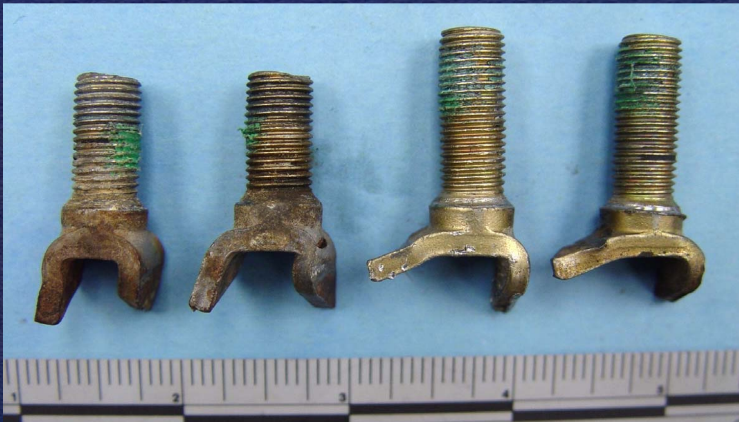
Seat attachment T-bolts from the accident
