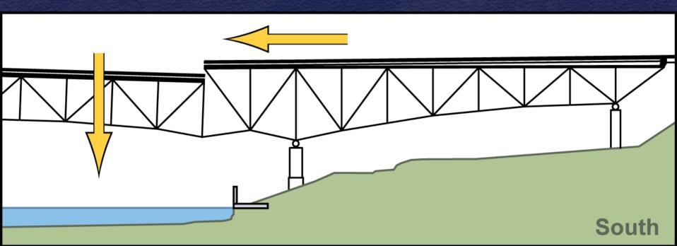
3. Other main truss members fractured in bending
