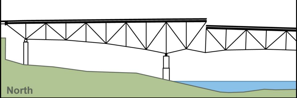
6. Deck truss collapsed above pier 8, causing loss of support for north approach spans, and this collapse spread southward toward pier 7
