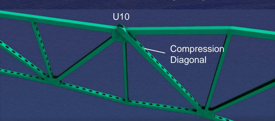
Dropping of center span created tension loading in main truss lower chords and secondary structural members. This loading pulled south portion of deck truss to the north, off pier 5, causing loss of support for south approach spans
