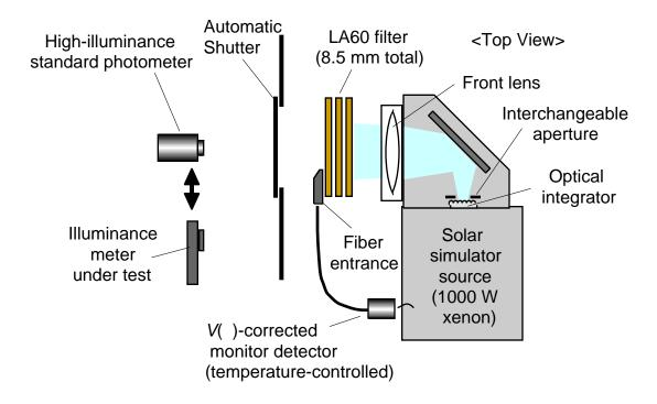
**Figure 2.** Configuration of the high illuminance calibration facility.
