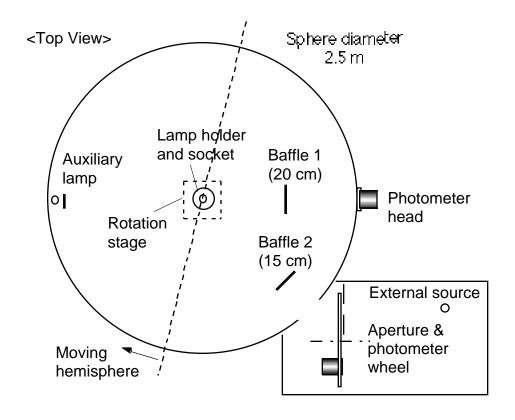
**Figure 5.** Arrangement of the new NIST 2.5 m integrating
