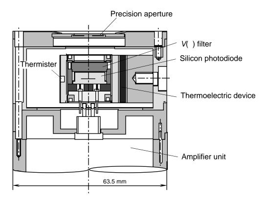
**Figure 3.** Design of the NIST temperature-controlled photometer used as high illuminance reference standards.
