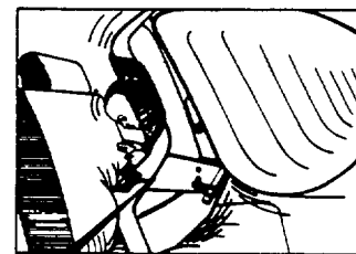
After the impact, the air bag could throw the safety seat up and into the headrest or between the seats.
