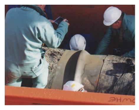
Figure 1. Buckle (raised area) in 40-inch-diameter steel pipe
