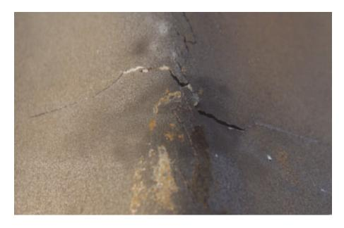
Figure 2. Close-up view of buckled area showing through-the-wall crack.
