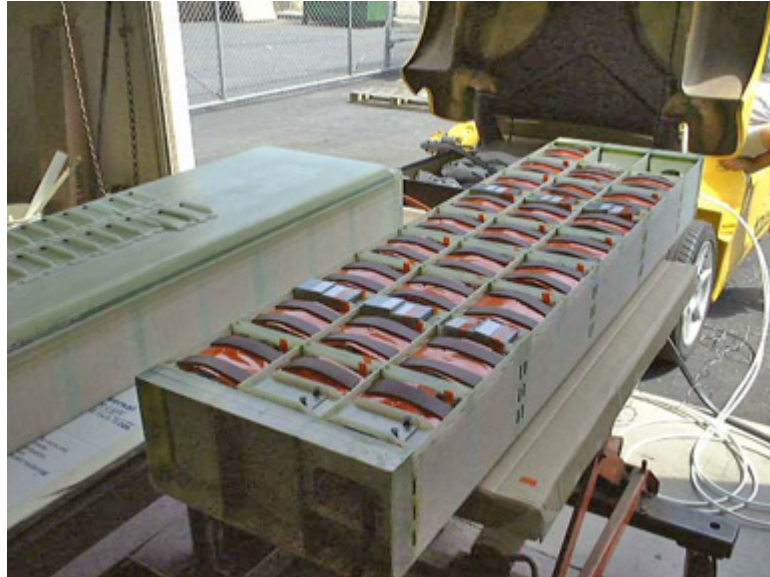
Figure 1. Approved battery pack in fiberglass case. The battery pack is without its cover and shows the modules secured in the fiberglass case.
