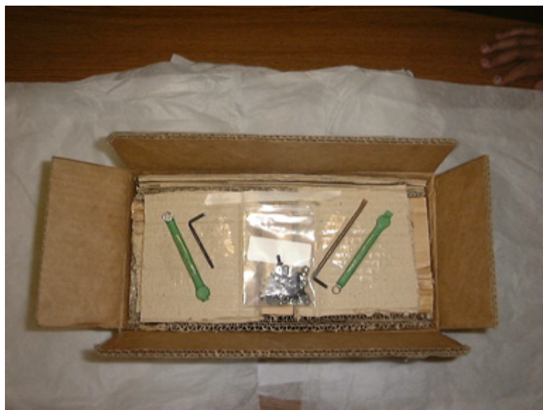
Figure 4. Tools taped to the top of the fiberboard lining covering the sample battery modules in figure 3, as was done with the accident package.
