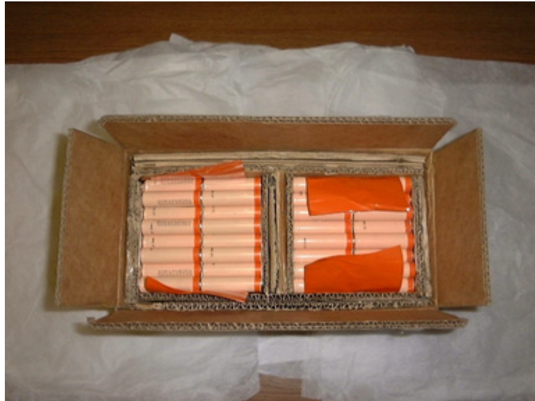
Figure 3. Sample modules in a 4G fiberboard box, as were the accident modules.
