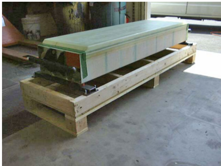
Figure 2. Approved battery pack in covered fiberglass case that is bolted to wooden base. (A wooden box that covers the fiberglass case is then secured to the wooden base.)
