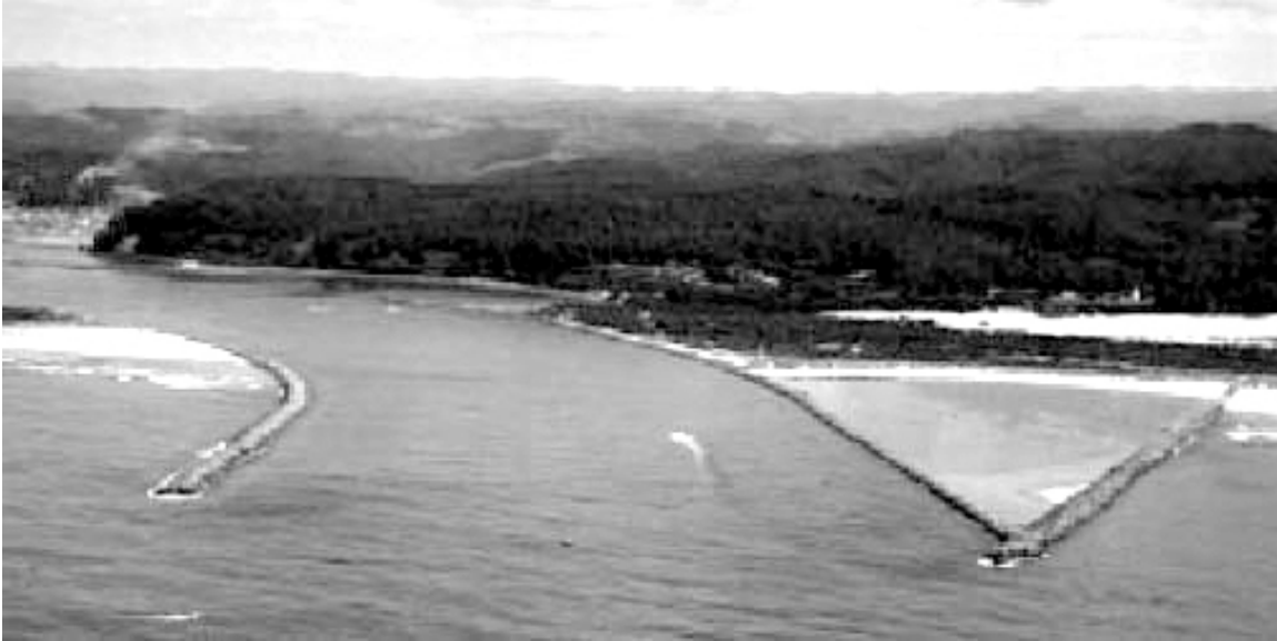
Figure. Looking east from the Pacific Ocean toward Winchester Bay, Oregon. North jetty is to the left of the photo, training jetty is to the right, and south jetty is to the far right. Photo courtesy Oregon State Marine Board, Boating in Oregon Coastal Waters < http://www.marinebd.osmb.state.or.us/CoastalWaters/Umpqua.htm >.
